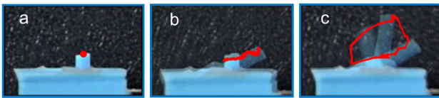
Figure 4 Asymmetric snapping actuator trajectories: (a) high resistance—no motion, (b) medium—reciprocal, (c) low—nonreciprocal
