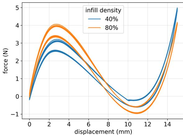
**Figure 3.** Force-displacement curves of the metamaterial with infill density 40% and 80%.
