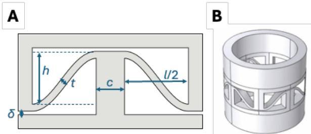
**Figure 1.** A) Design parameters of the metamaterial unit cell in plane. B) CAD design of the final metamaterial with cylindrical topology.
