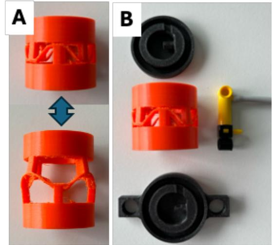
**Figure 2.** A) Metamaterials in the two stable states. B) Components of the bistable actuators: metamaterial, single-acting cylinder, and holders.
