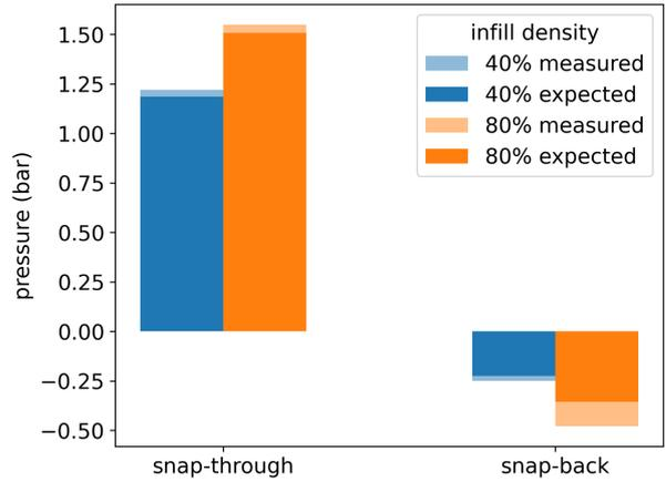
**Figure 4.** Snap-through and snap-back pressures of the actuators featuring the metamaterials with infill density 40% and 80%, both measured and expected from the force-displacement curves.
