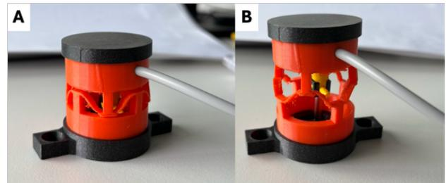
**Figure 4.** The bistable pneumatic actuator in the two stable configurations: the designed (A) and the metastable (B) ones.
