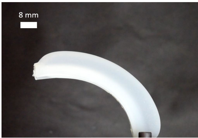
Fig. 7. Bending deformation for a cilium with length 57 mm at a pressure of 50 kPa.
