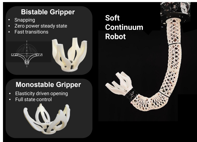
Fig. 1. Overview of the developed bistable gripper and the monostable design for comparison, together with its integration on the Helix soft continuum manipulator.
