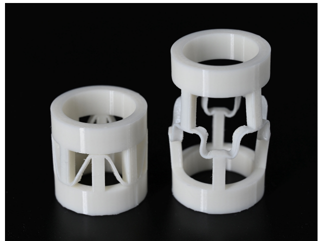
Figure 1 3D printed sample of the NC-clutch in closed (left) and open (right) state
